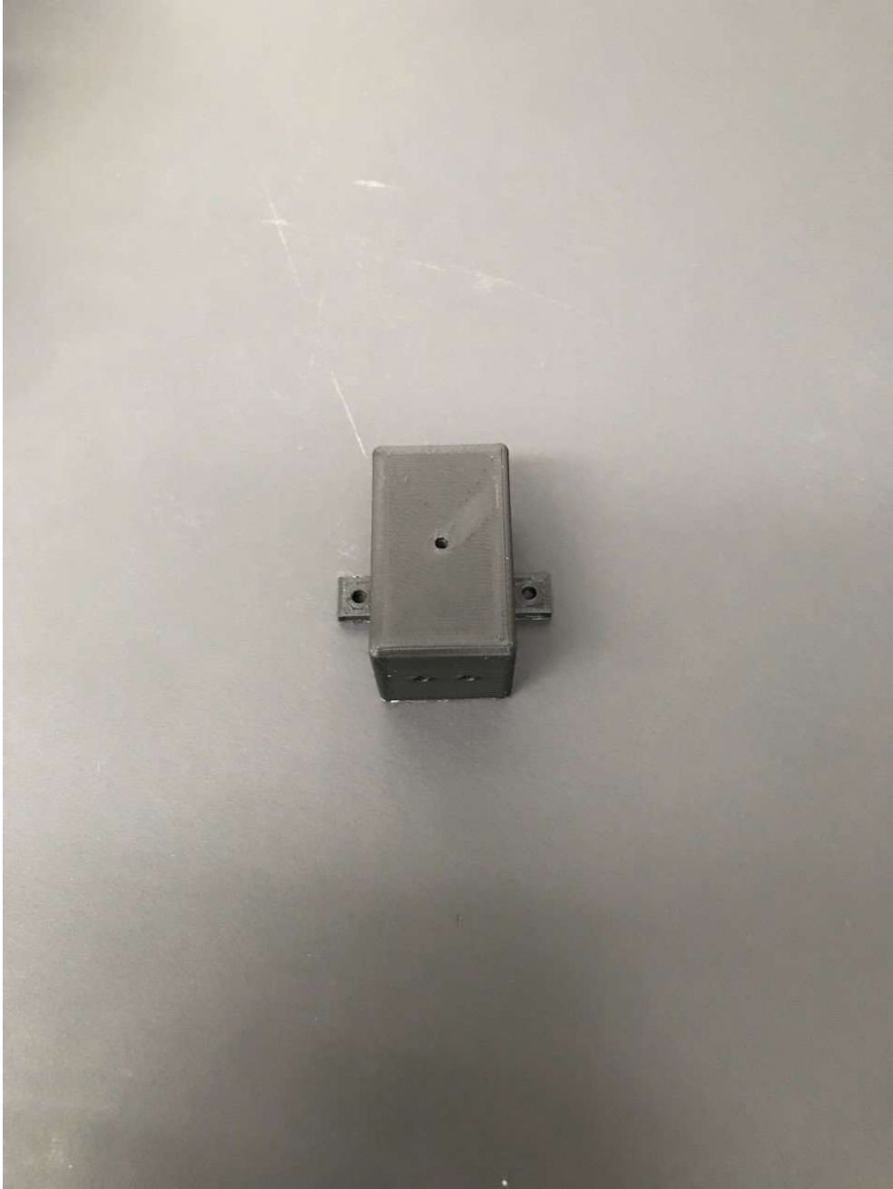
Figure 2 - Prototype part 2 – Wifi-module and resistance sensor
